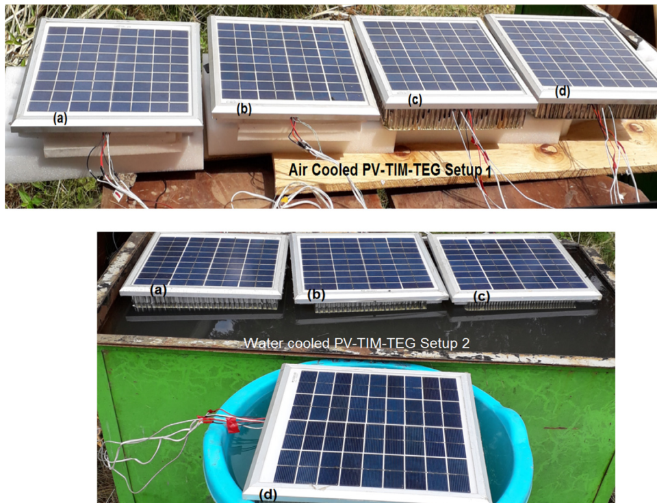
Fig. 6. Air- and water-cooled PV-TIM-TEG setups 1 and 2 (a) graphite (b) heat spreader (c) aluminium foil (d) bare cells.
